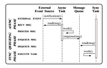
Figure 3: Collaboration between Layers in the Half-Sync/Half-Async Pattern
