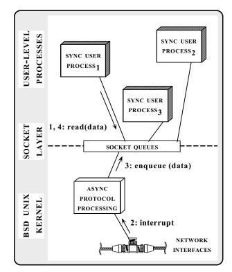
Figure 1: BSD UNIX Software Architecture
