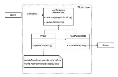
Fig. 7. Application of a Proxy in DASH
