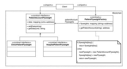
Fig. 6. Applying the Flyweight Registry Model to DASH
