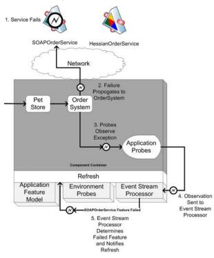
Each feature in the feature model that could potentially fail is associated with a group of event stream queries. At runtime, when a query associated with a feature returns a result, Refresh is notified that the associated feature has failed, as shown in Figure 7. The data and objects observed and analysed by Refresh are determined by the query specifications.
