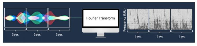
Fig. 1. To standardize input into the neural network, acoustic signals were segmented into 3-second chunks (left) and transformed into spectrograms using the Fourier transform (middle). Spectrograms displayed frequency over time, with intensity coded by grayscale (right).
