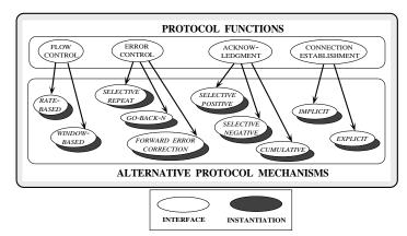
Figure 2: Protocol Functions and Protocol Mechanisms
