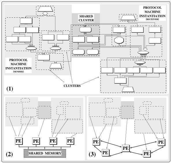
Figure 12: Clustering and Mapping Protocol Resources onto Multi-Processing Platforms
