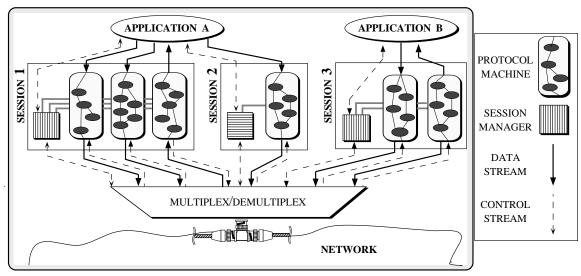
Figure 3: Relationship between Entities in the Function-based Communication Model
