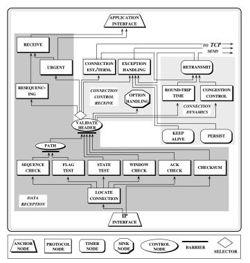
Figure 6: A Flowgraph for the TCP Receiver Protocol Machine
