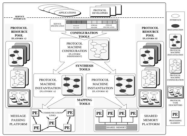
Figure 11: Resources and Tools used during Protocol Generation and Execution
