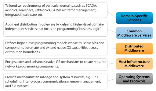
Figure 12. Key layers of distributed CPS software infrastructure.
