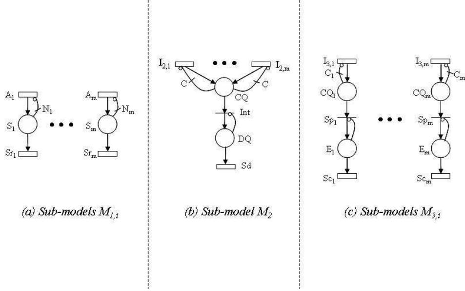
Figure 3: Model decomposition in SRN
