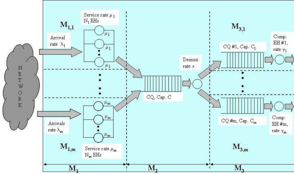
Figure 1: Queuing model of an asynchronous Web server
