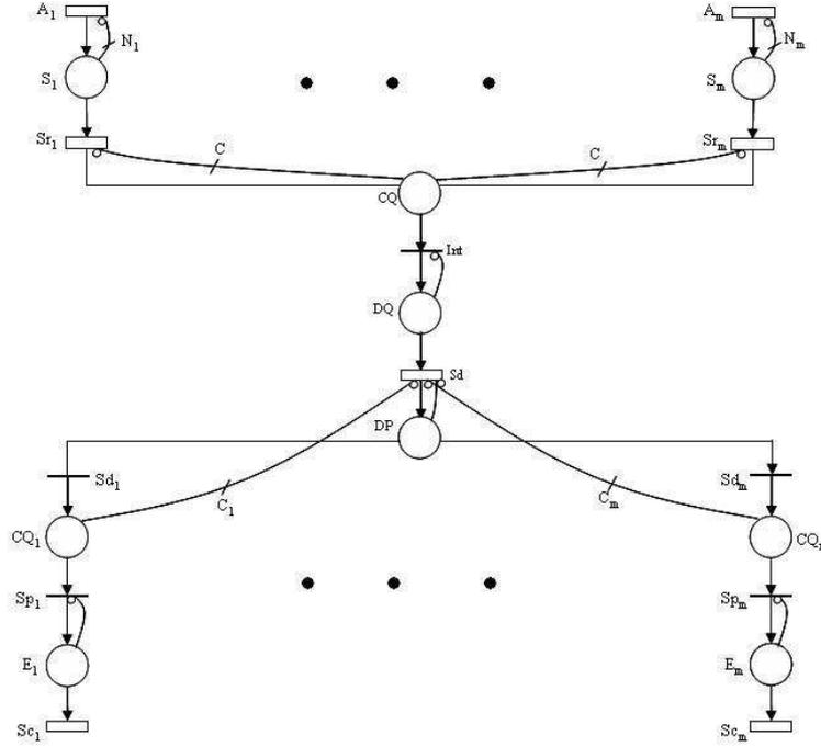
Figure 2: SRN implementation of the queuing model
