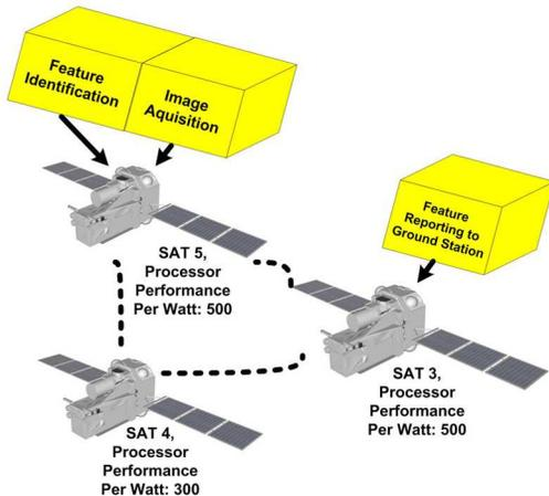
(b) A Software Deployment Topology for the Fractionated Spacecraft with Superior Performance per Watt
