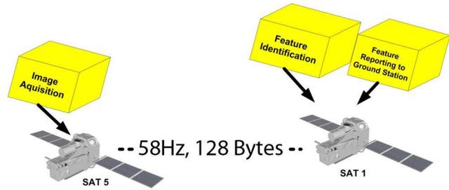
(a) A Software Deployment Topology Using Two Nodes
