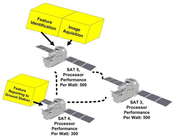
(a) A Software Deployment Topology for the Fractionated Spacecraft
